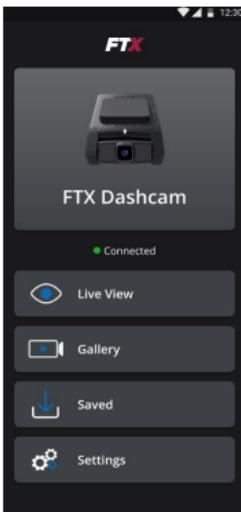
Manual Connect is required for the initial setup. Find the FTX's Wi-Fi network on your phone's Wi-Fi network list and connect by using the password "12345678", then return to the App.
